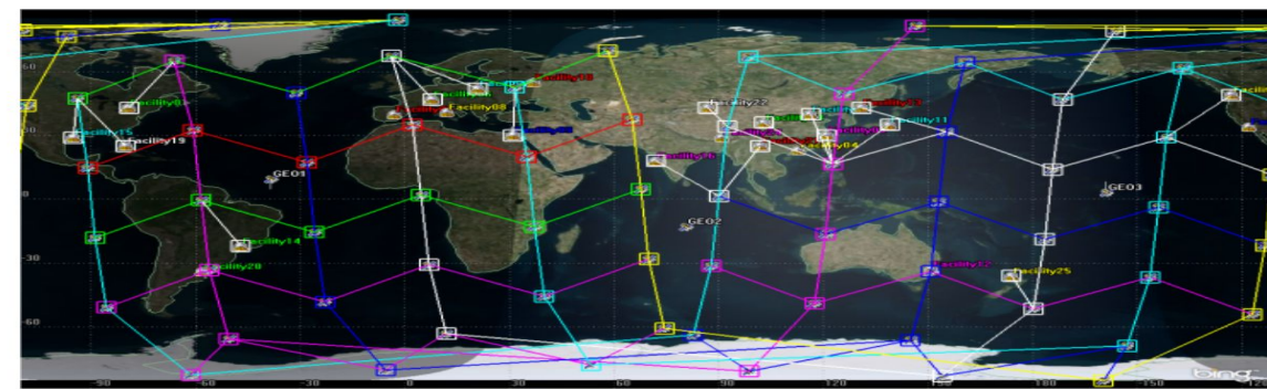
FIGURE 6. Satellite network topology used in simulation. (Picture from STK.) Considered ISL are drawn in the picture.
